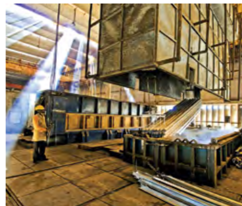
Galvanizing in progress
