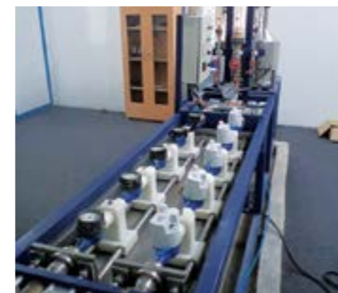
Testing of water meters
