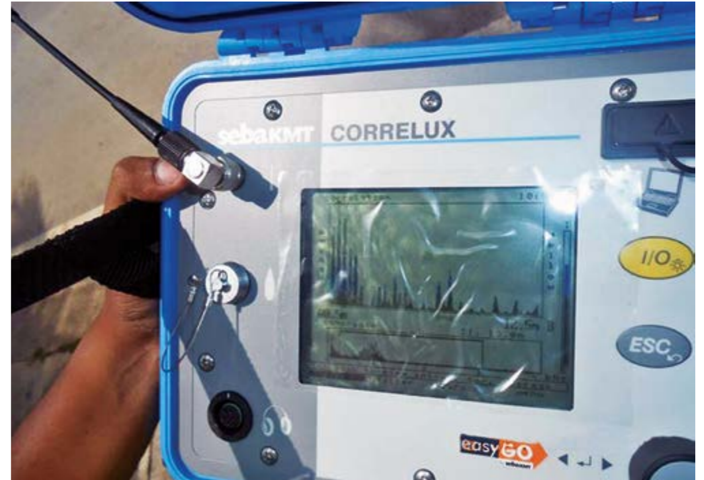
Leak detection and rectification
