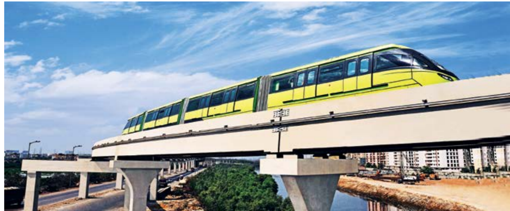
Mumbai Monorail - India's first 750 V DC traction based urban transit system
