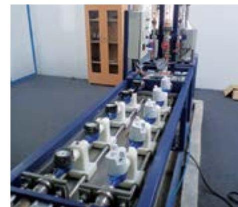
Testing of water meters
