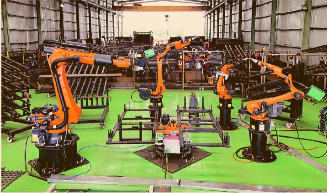
TOP SPEED: (Left) Robotic arms at a L&T factory assemble structures to be used for the Mumbai-Ahmedabad bullet train. (Top) Bridges for the train are being built based on surveys that use laser pulses to analyse the Earth's surface. (PHOTOS: L&T)
